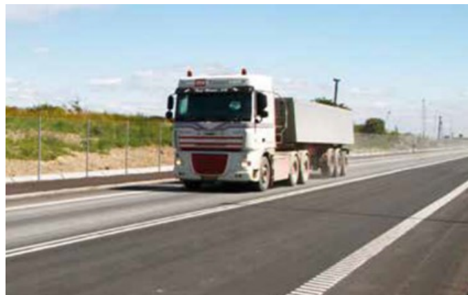
Test of bottom ash gravel at Nordsøvej in Copenhagen from 2012 to (so far) 2022 (AFATEK).
