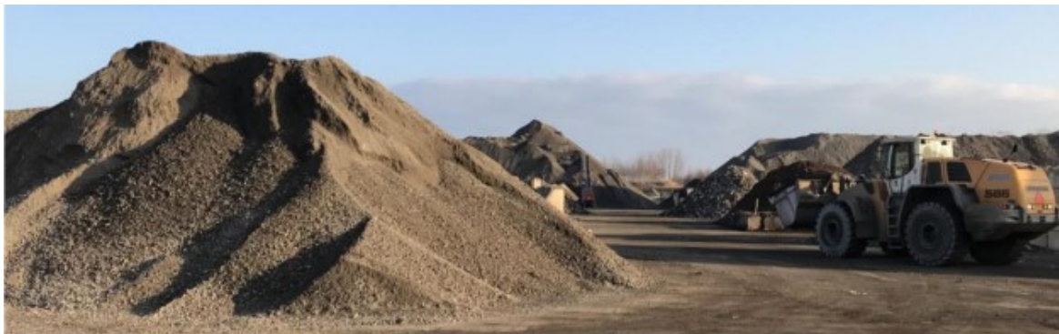
Processed bottoms – certified bottom ash gravel, ready for use (AFATEK).
