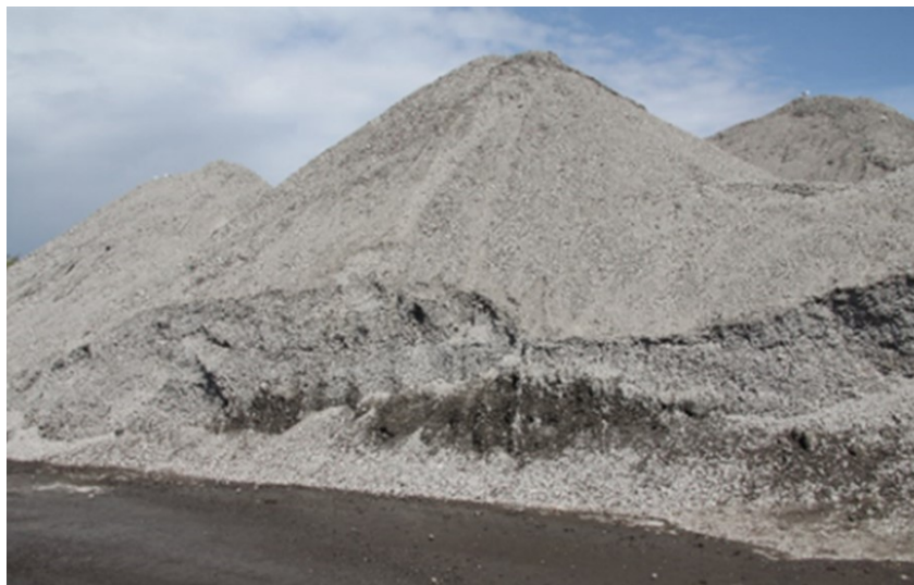
Maturation of the bottom ash gravel for 2 – 3 months dries the ash to a moisture content of 10 – 12 % which is sufficient to allow effective removal of metals. The bottom ash gravel also takes up CO 2 during maturation.
