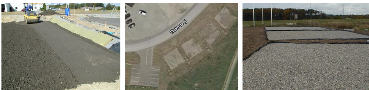
Photos from the demonstration site for utilisation of bottom ash gravel at Ydernæs in 2002 - 2019 (DanWS).
